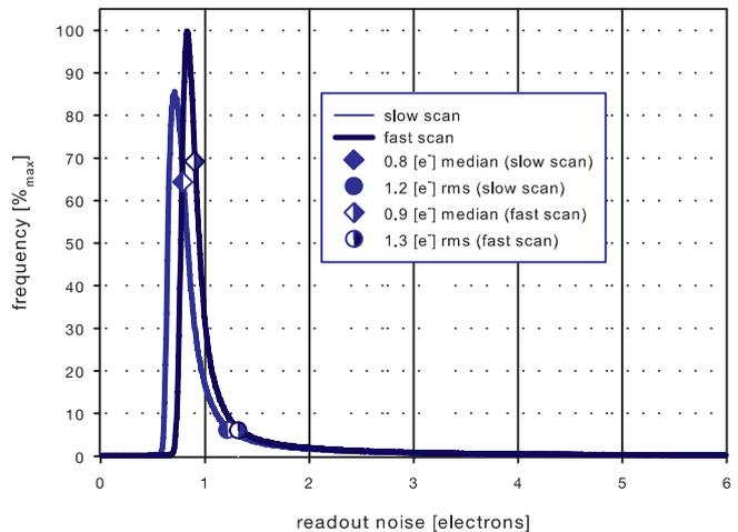
Noise distribution of the rms raw data values (noise filter off) of each pixel in the dark image of a pco.edge 4.2 at different readout speeds (slow scan / fast scan).
