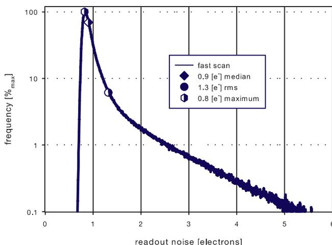
The left figure shows the same fast scan curve of the pco.edge 4.2 only in a logarithmic y-axis (frequency) scaling, to emphasize that most of the pixels have an average readout noise in time that is smaller than 1 electron and there are few pixels (less than 1 % of the maximum), which have a readout noise of 3 – 6 electrons.
