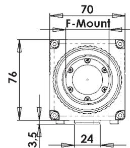
All dimensions are given in millimeter.
